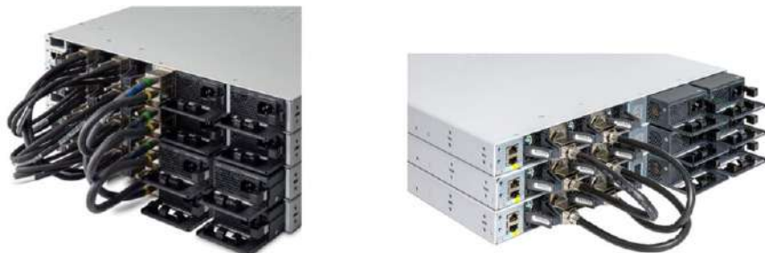
Figure 4. Cisco Catalyst 9300 Series modular uplink models stack (C9300 SKUs) and fixed uplink models stack (C9300L SKUs)
